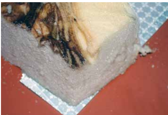
^ Sample of foam from cavity
