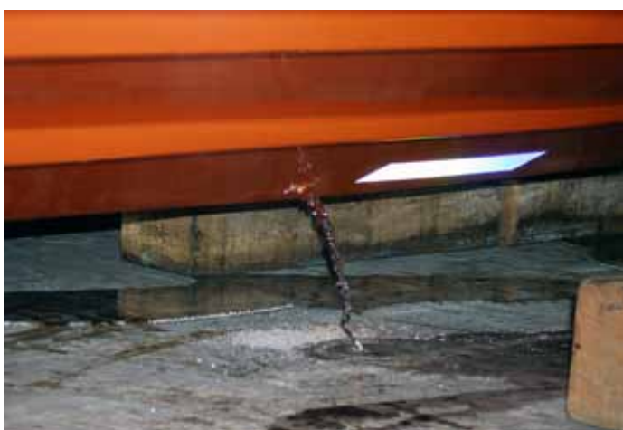
^ Water draining from trapped compartment
