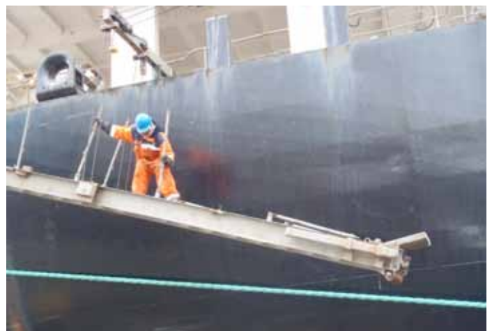
^ Rigging an accommodation ladder – no safety harness or fall prevention device in use – this is not a safe practice
