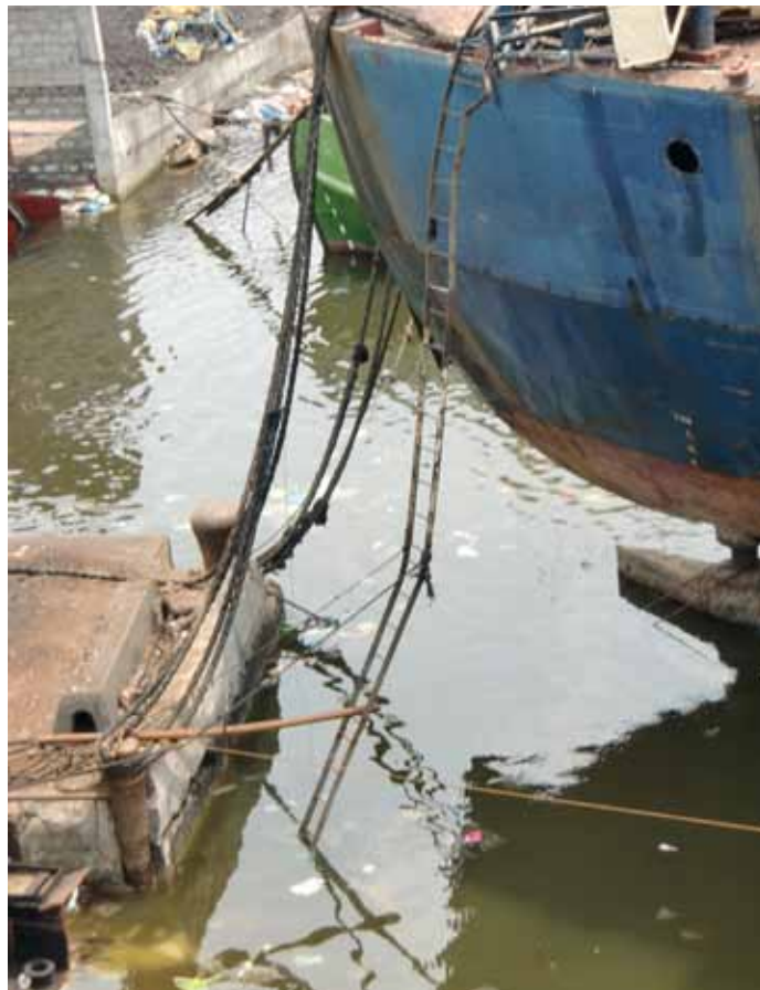
^ Ladders should not be used as a means of safe access to ships – this is not a safe practice
