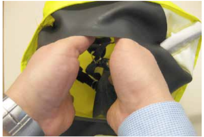
^ Mask hood and neck-tightening rubber membrane inadequate
