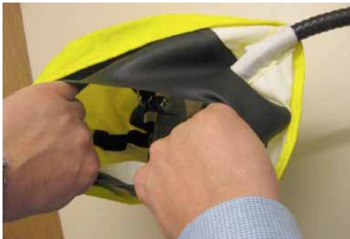
^ Mask hood and neck-tightening rubber membrane inadequate
