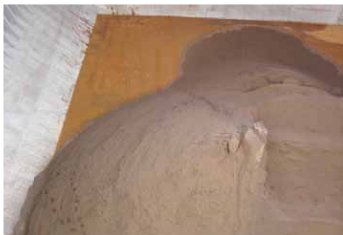
^ Signs of water in the cargo hold during loading of sinter feed ore at Santana, Brazil
