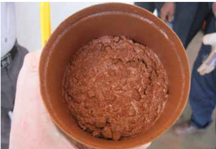
^ Can test showing a sample of iron ore fines with signs of water
