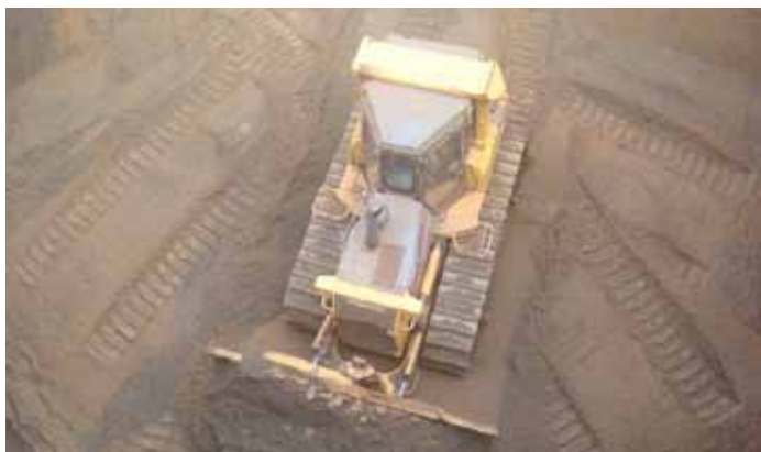
^ Bulldozer trimming sinter feed ore inside a cargo hold at Santana, Brazil
