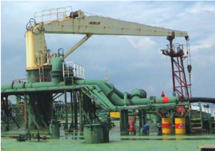
^Hose handling crane – driver unable to see over ship's side
