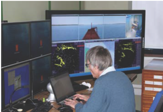
^ Modern ECDIS usually incorporates additional electronic navigational systems (image courtesy of Warsash Maritime Academy)
