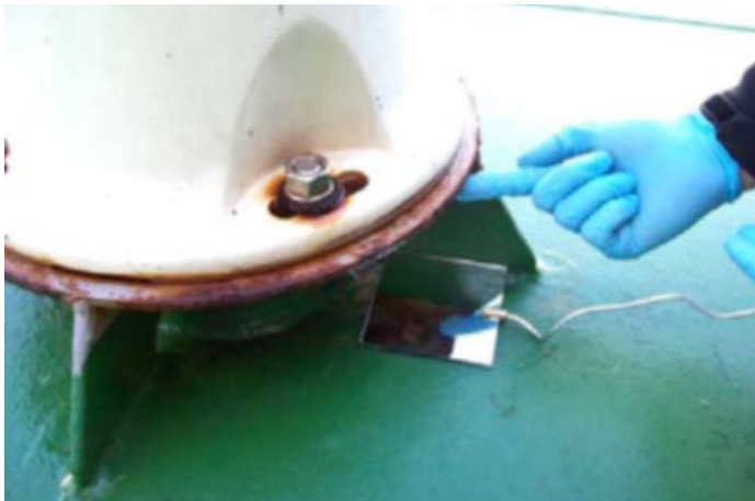
^ Mirror on a stick To look around corners and under edges.
