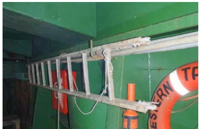
^ Portable ladder badly stowed, and is blocking safety equipment
