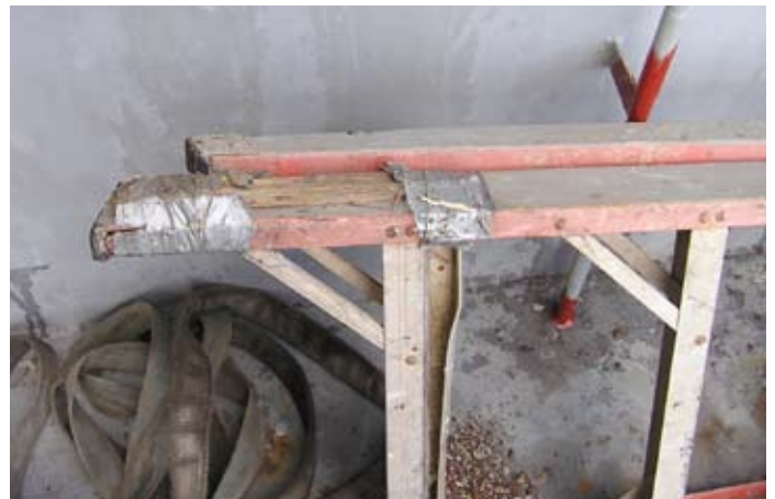
^ Poorly maintained and damaged portable ladder. This ladder should be removed from use and disposed of
