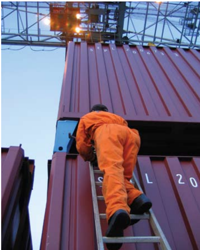
^ Example of poor safety when using a portable ladder
