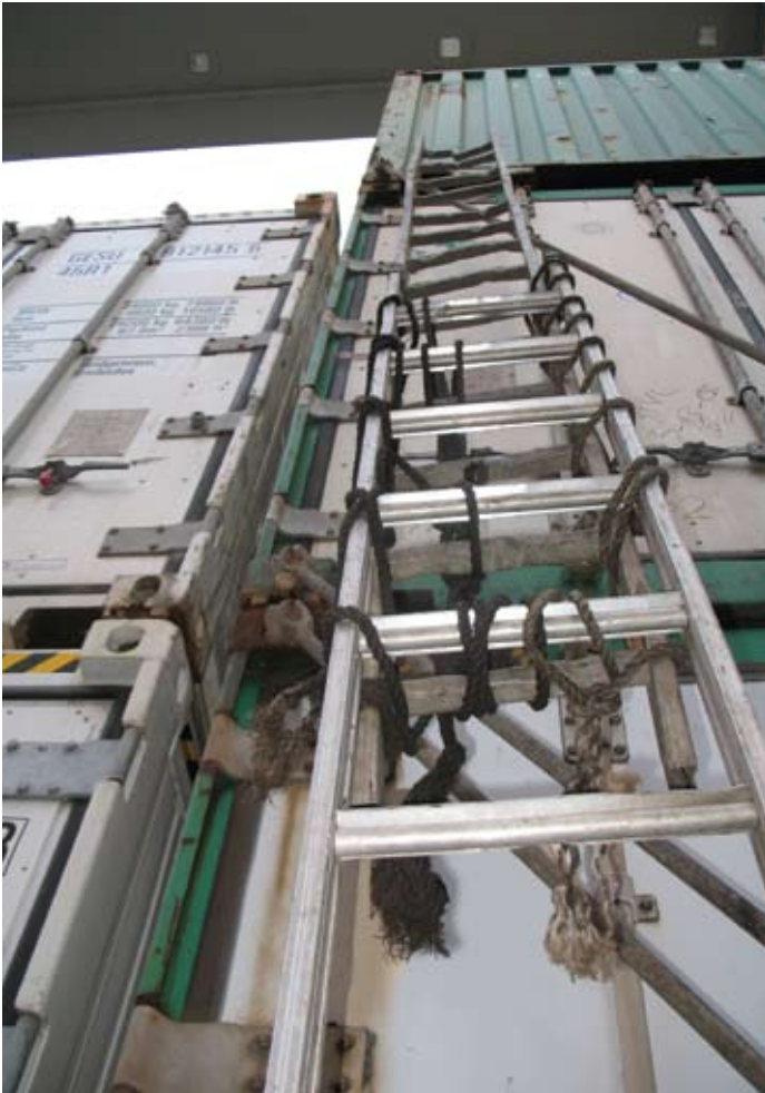
^ A severely damaged portable ladder beyond repair. This ladder should not be used
