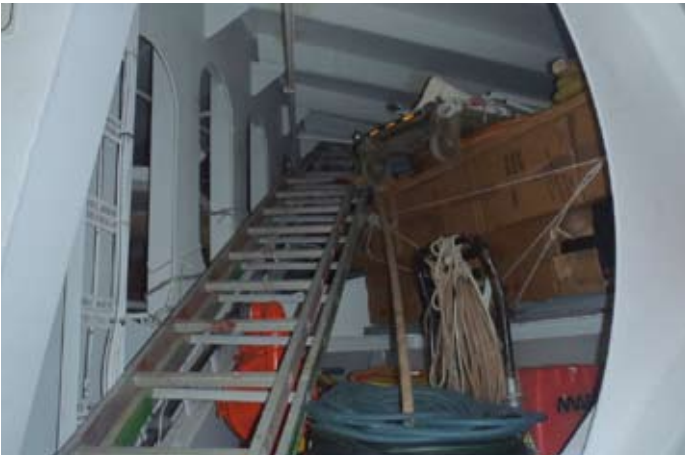
^ Portable ladders stowed incorrectly in a forecabin store
