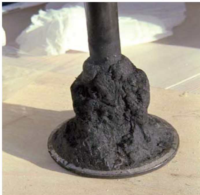
√ Figure 3: Exhaust valve carbon build-up
