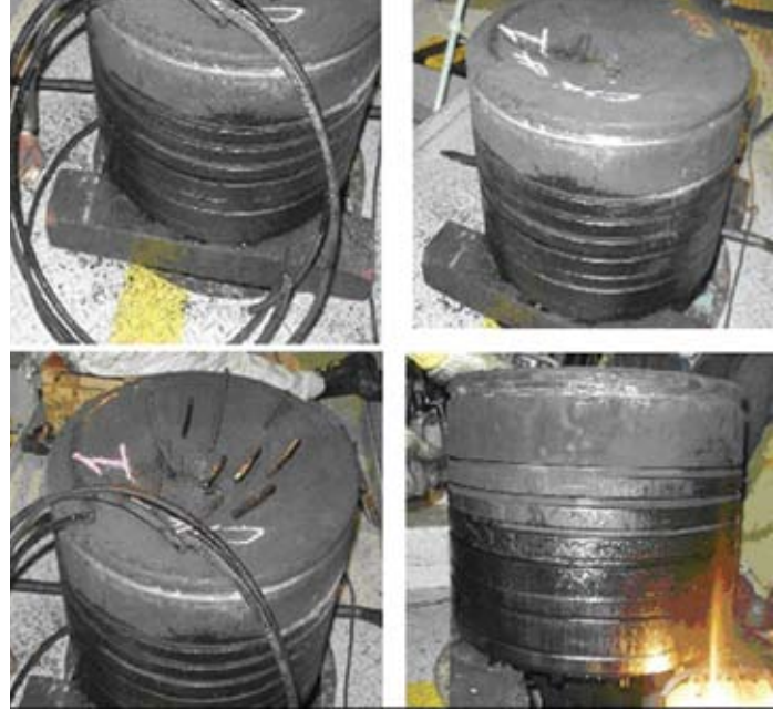
vFigure 2: Piston damage due to poor quality HFO
