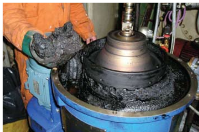
√ Figure 1: Heavy sludge contamination
