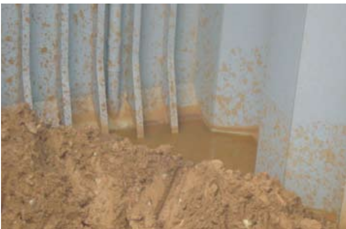
^ Water found during loading of nickel ore cargo
