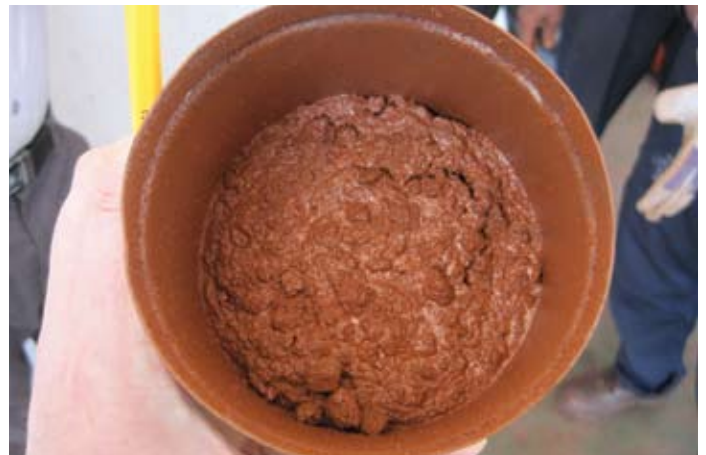
^ Can test showing moisture on surface
