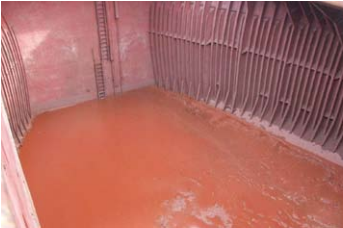
^ Cargo hold with wet iron ore fines. Photo courtesy of Brookes Bell
