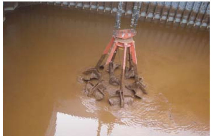
^ Discharging wet iron ore fines
