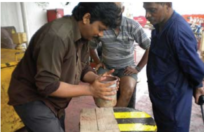
^ Can test conducted by shore side workers.
