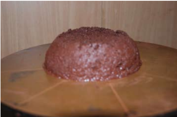
^ Cargo sample on flow table. Photo courtesy of Brookes Bell.
