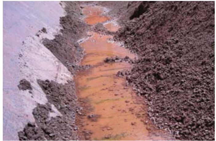
^ Water draining from iron ore fines. Photo courtesy of Brookes Bell.
