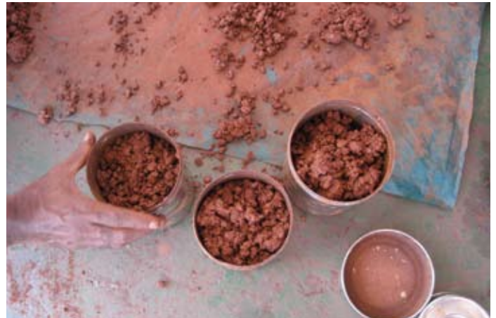
^ Separate can tests. Photo courtesy of Brookes Bell.
