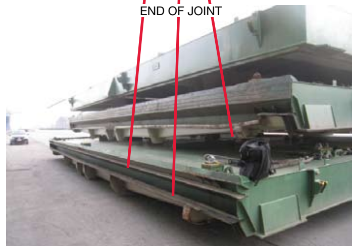
^ This picture and diagram shows a pontoon hatch cover arrangement that would most likely fail an ultrasound hatch cover test. Even with foam and tape, this arrangement is likely to allow water ingress into a hold sufficient to damage water-sensitive cargo when the ship is experiencing heavy weather
