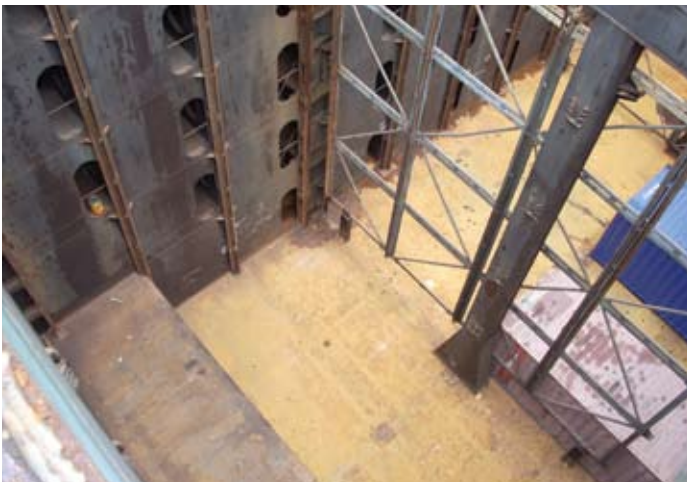
^ This container hold may be suitable for general cargo. It would depend on the cargo and the hatch cover condition
