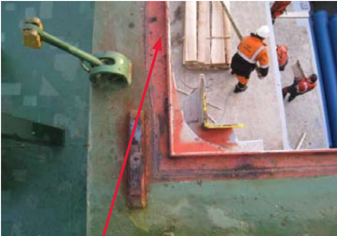
^ View of area where CAT seal acts on the coaming table
