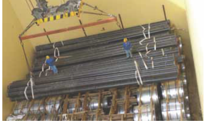
Pipes loaded on top of steel coils.
