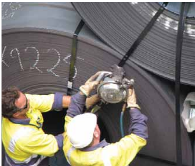
Steel bands are pneumatically tightened.
