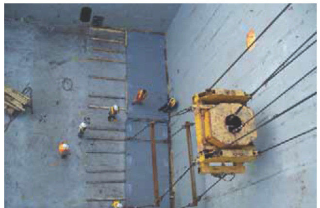
Steel plate is stowed fore and aft on athwartship laid dunnage in a square-sided hold.
