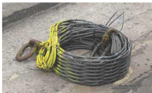
Coils are loaded with ribbon slings.
