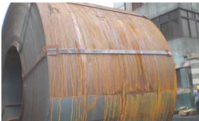
Condition of coils at discharge port - rusted.
