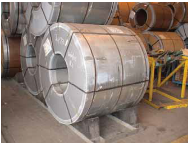
Coil prior to stowage correctly wedged.
