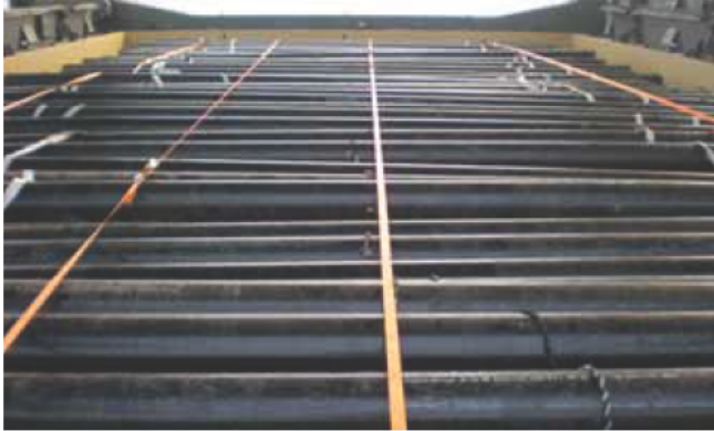
Pipes secured in the hold, but lashings are of little value.
