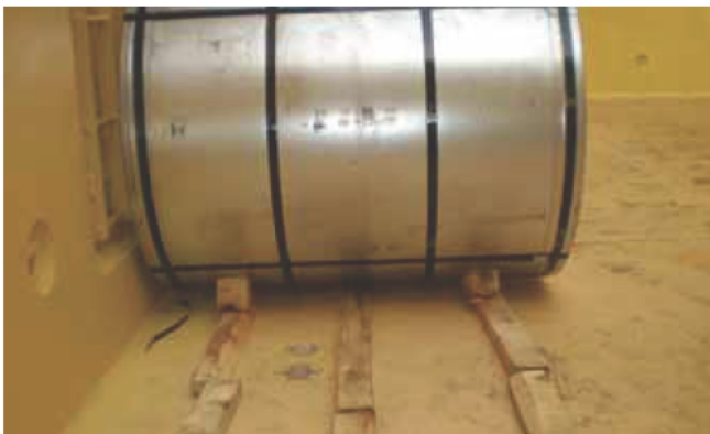
Coils wedged in position.
