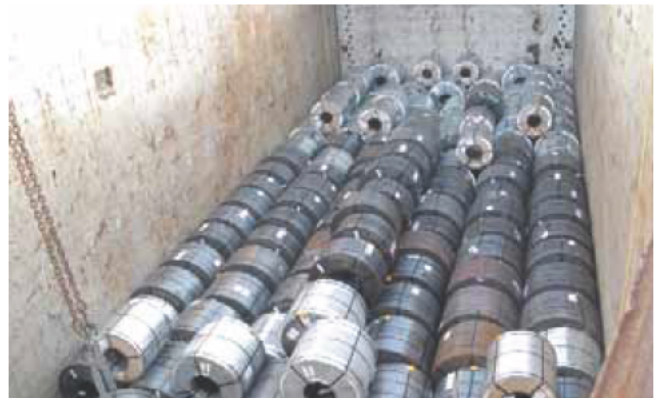
Coils tightly stowed with centre line key coils and multiple key coils fore and aft.
