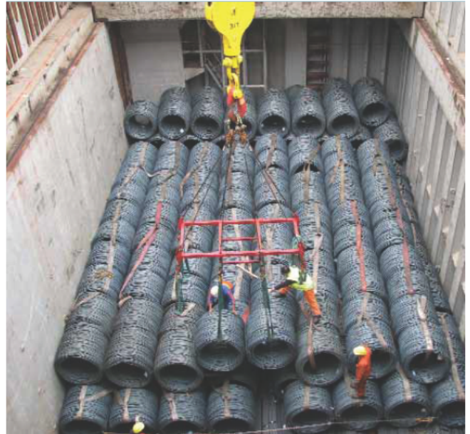
Coiled wire rod correctly stowed in a square hold.
