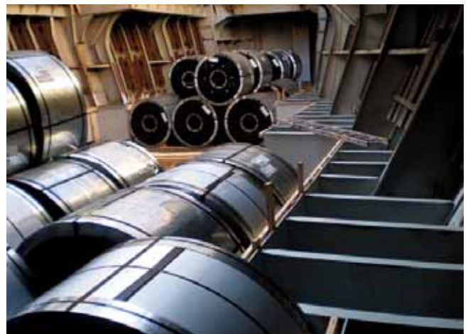
No.1 hold is 'squared off' with a steel structure.
