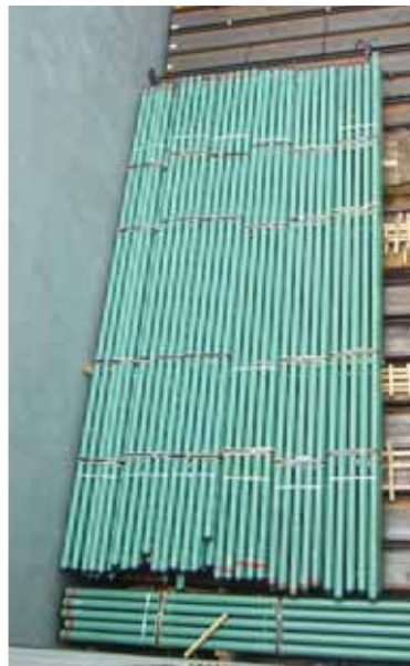
Pipes are stowed fore & aft and athwartships. Dunnage has not been placed between the pipes stowed athwartships and the ship's side bulkhead.
