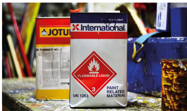
Figure 5: Fuel source stored above flashpoint temperature
