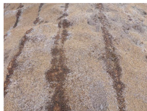
Drip lines on cargo surface from ships sweat
