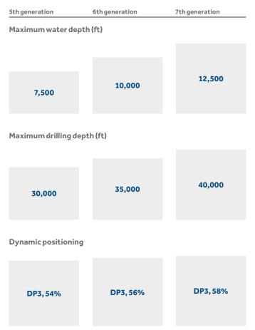
Figure 2 – Development of floating MODU designs. Source: CRSL
