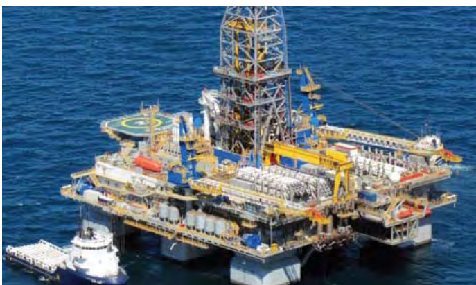
Semi-submersible Drilling Unit (Noble)
