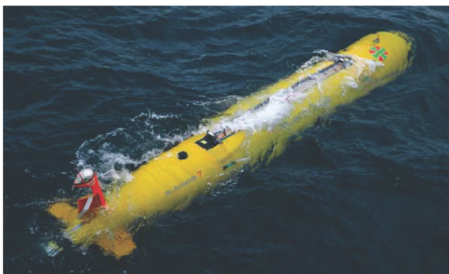
SUBSEA 7'S GEOSUB AUV PERFORMING THE WORLD'S FIRST PIPELINE INSPECTION
