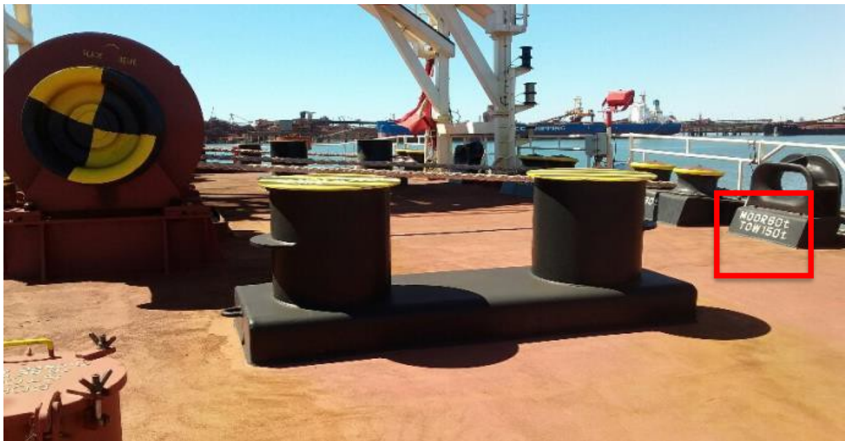
Figure 3: SWL markings on vessel deck fitting
