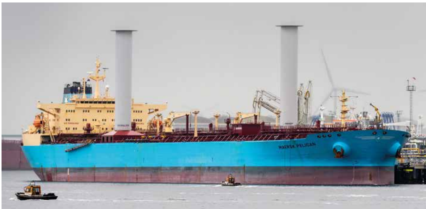
Crews need to understand fuels and propulsion means of the future including Flettner rotors, shown here on the Maersk Pelican
