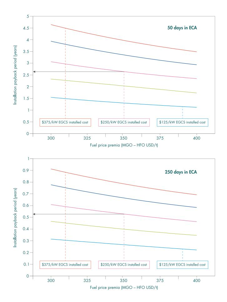
Figure 52: Illustration of payback for an Exhaust Gas Cleaning System (Equipment and initial installation)
