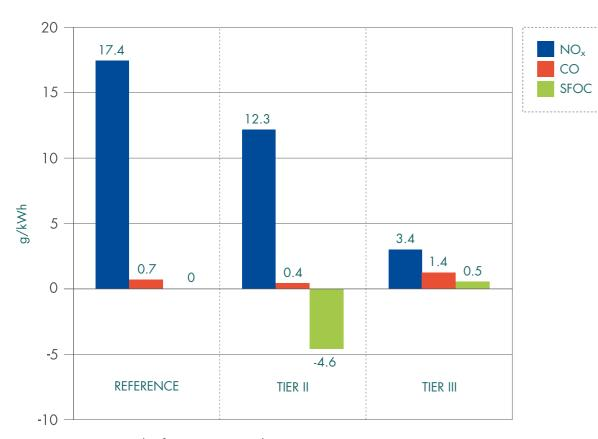
Figure 37: Results of EGR tests on 2-stroke test engine adjusted to achieve Tier II & Tier III compliance. (Power for the EGR blower is not included in Specific Fuel Oil Consumption values. Other emission values (PM, HC) remain basically unchanged)
