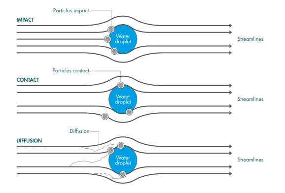
Figure 31: Particle trapping process
