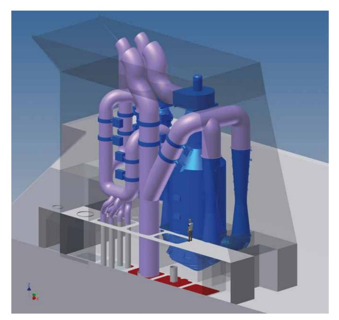
**Figure 42: Multi-stream exhaust gas cleaning unit** (2 inlet quench sections can be seen at the right and an ID fan at the top of the exhaust gas cleaning unit)
