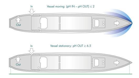
Figure 12: Measurement of position pH - Method 1
