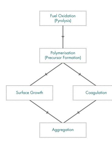
Figure 4: Particle formation – diesel engine fuel combustion
