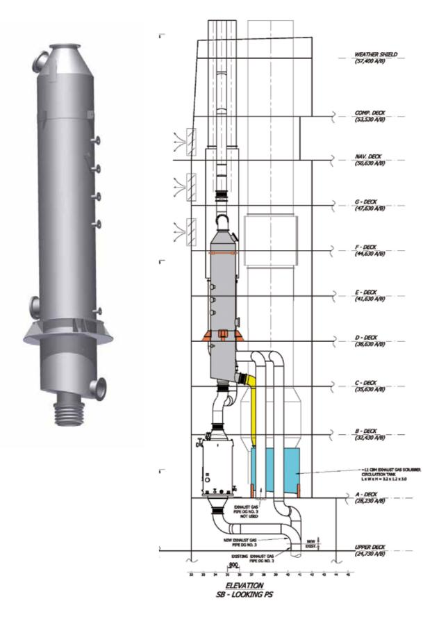
Figure 49: Exhaust gas cleaning unit arrangement – container vessel (Hybrid scrubbing system - 3.5MVV auxiliary engine. Note position of circulation (process) tank is above the vessel's upper deck)
