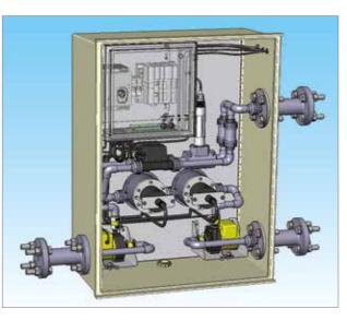
**Figure 15: Washwater monitoring instrumentation cabinet** (From bottom to top, left to right: sampling pumps, turbidity and PAH sensors, flow and pH sensors, control electronics)
