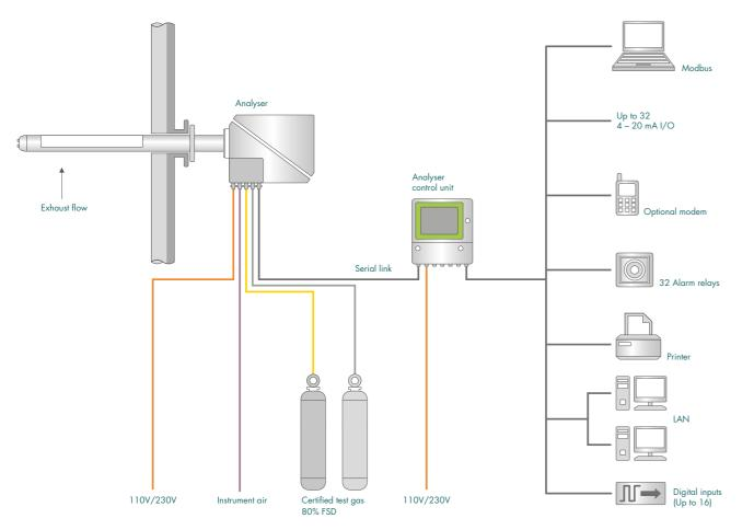
Figure 46: In-situ CEMS arrangement
