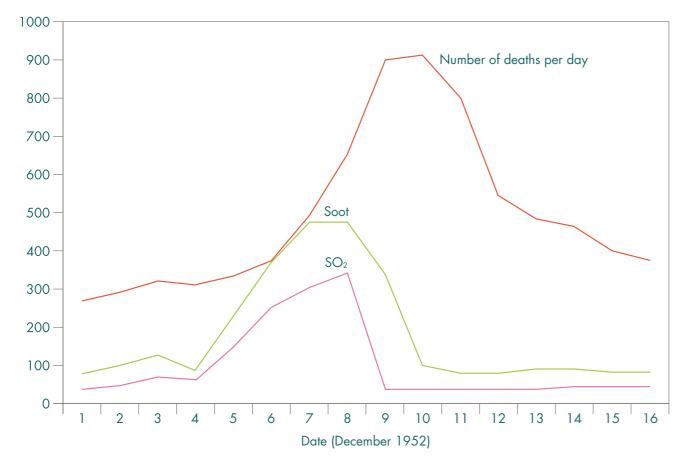
Figure 1: The link between atmospheric sulphur dioxide concentration and human mortality
