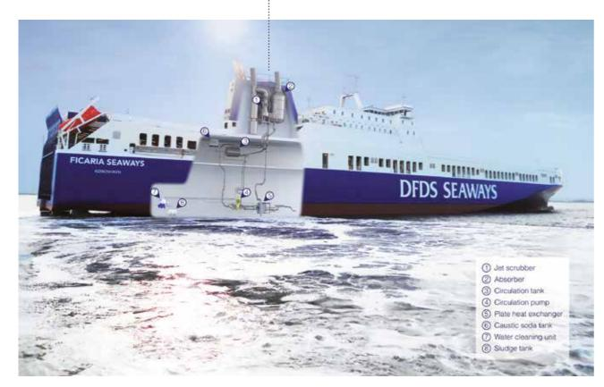
**Figure 48: Exhaust Gas Cleaning System arrangement – RO-RO** (Hybrid scrubbing system - 21MW slow speed main engine) Courtesy Alfa Laval
