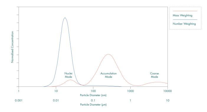
Figure 7: Graph of bimodal range of PM for diesel engines
