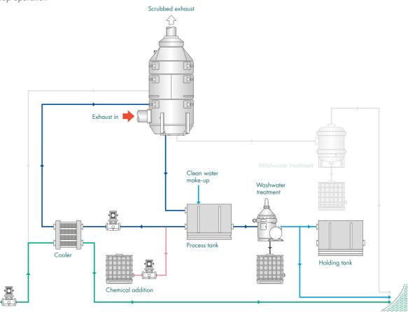
Figure 21: Hybrid Exhaust Gas Cleaning Systemclosed loop operation
