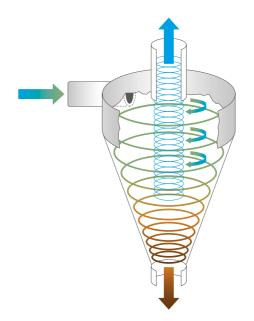
Figure 25: Hydrocyclone schematic
