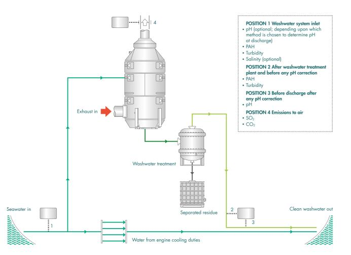
Figure 24: Position of water quality and emissions monitoring instrumentation
