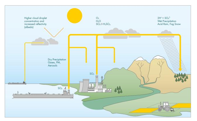
Figure 2: Sulphur oxide deposition without exhaust gas cleaning
