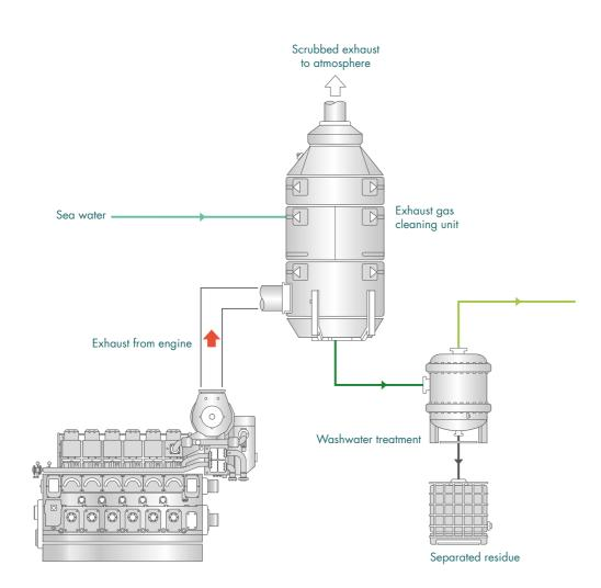
Figure 17: Exhaust Gas Cleaning System basic components (See Figure 24 for position of instruments)
