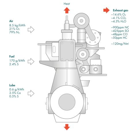
Figure 11: Typical exhaust gas compositionslow speed two stroke engine using residual fuel
