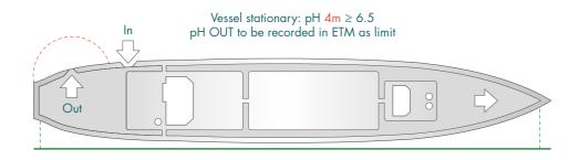
Figure 13: Measurement of position pH – Method 2
