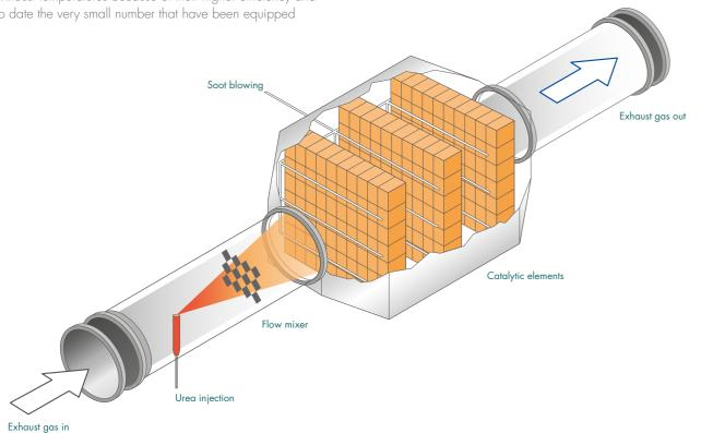
Figure 36: Selective Catalytic Reduction unit Courtesy Wärtsilä
