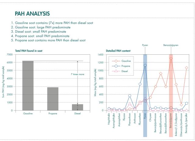
Figure 3: PAH analysis, gasoline, diesel, propane Courtesy Dr. Lianpeng Jing, Jing Ltd <sup>[97]</sup>
