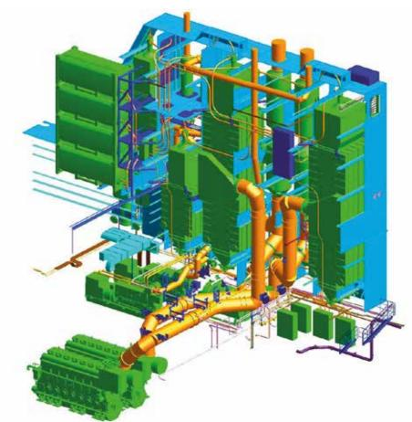
Figure 29: Arrangement of dry exhaust gas cleaning for multiple engines (Exhaust gas cleaning units for the 2 main engines are forward (right) and middle of the funnel casing. Smaller exhaust gas cleaning units for the 2 auxiliary engines are middle and aft (partly obscured). Granulate storage containers can be seen aft, in the top foreground. Total engine power 22MW.)
