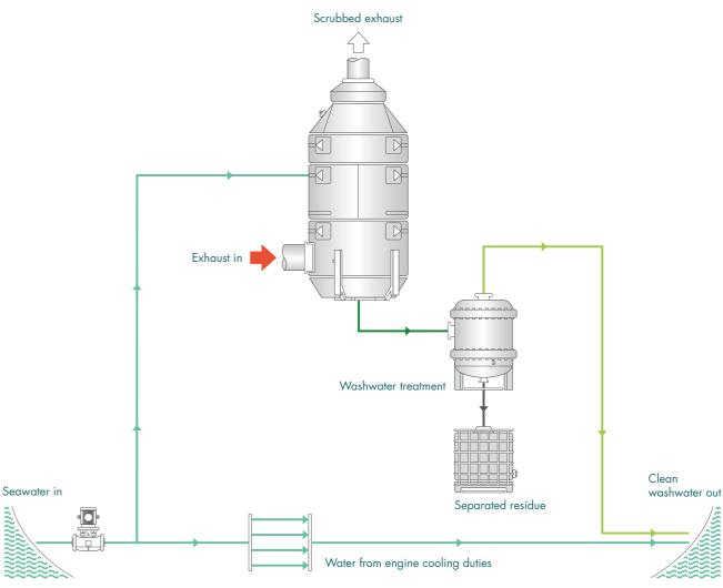
Figure 18: Open Loop Exhaust Gas Cleaning System
