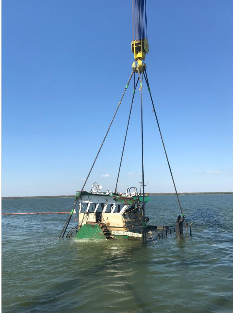
Lifting of a tug submerged during Hurricane Harvey
