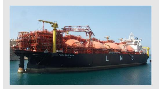
No Carriage of Cargo, permanently moored and 'production' of Gas from Liquid
