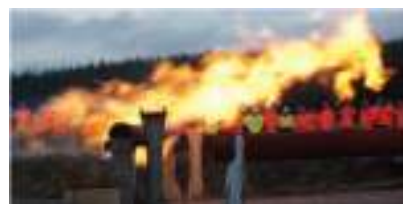
Pool Jet Fire – NG leak from 20mm hole at 70barg
