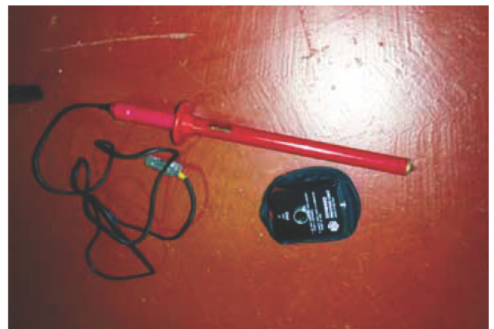
^ Example of approved 'Potential Indicator' (or earthing rod)
