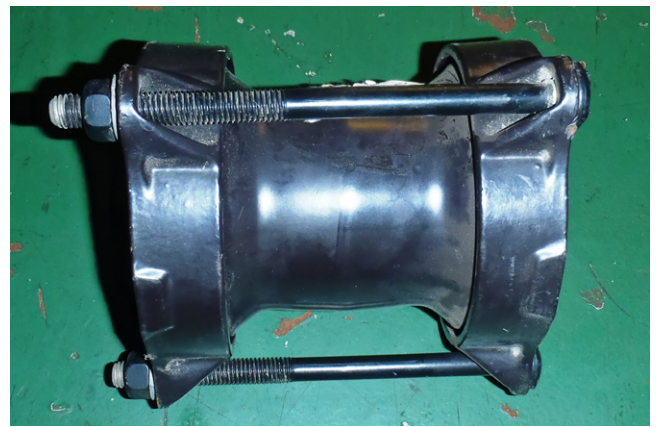
Figure 19: Slip type coupling
