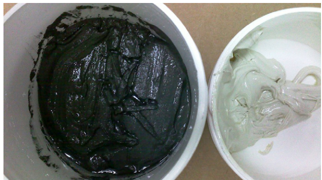
Figure 15: Plastic steel before mixing
