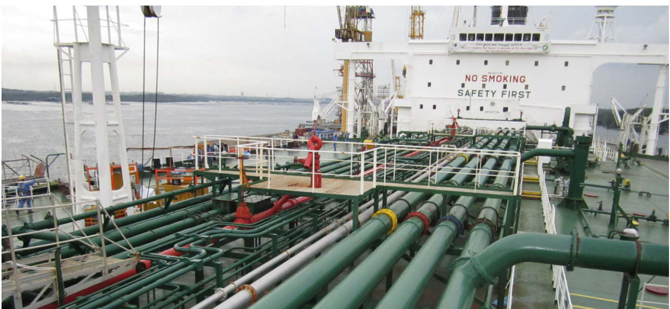
Figure 2: Typical cargo piping
