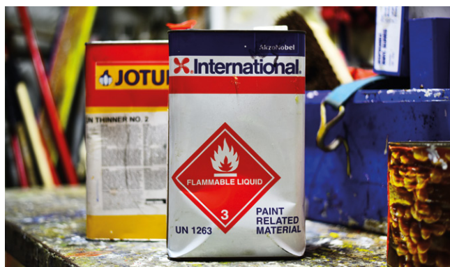
Figure 5: Fuel source stored above flashpoint temperature
