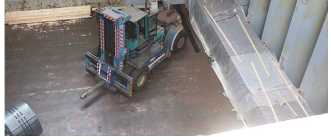
Figure 46: Coils being stowed by a forklift fitted with a single round tine
