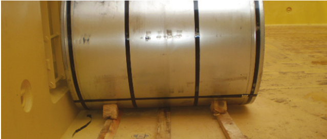
Figure 45: Coils wedged in position
