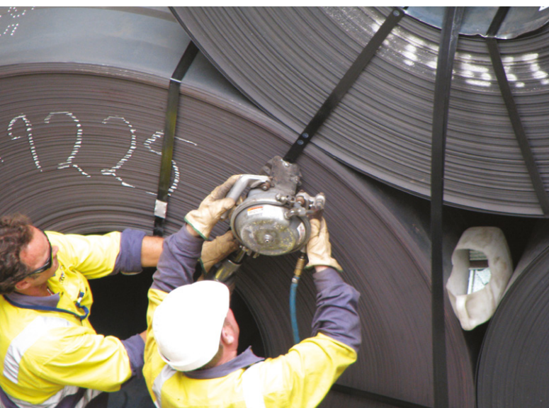
Figure 33: Steel bands are pneumatically tightened
