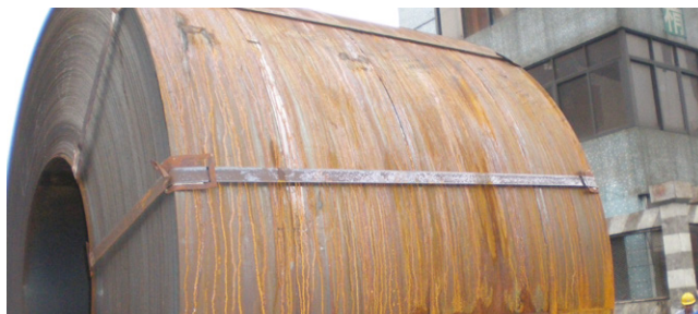
Figure 50: Condition of coils at discharge port – rusted
