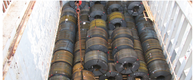
Figure 48: Coils dropped straight into the hatch square. Note use of wire ribbon slings
