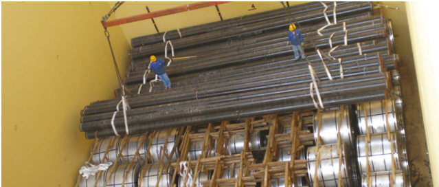
Figure 44: Pipes loaded on top of steel coils
