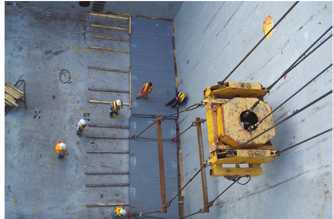
Figure 28: Steel plate is stowed fore and aft on athwartship laid dunnage in a square-sided hold.
