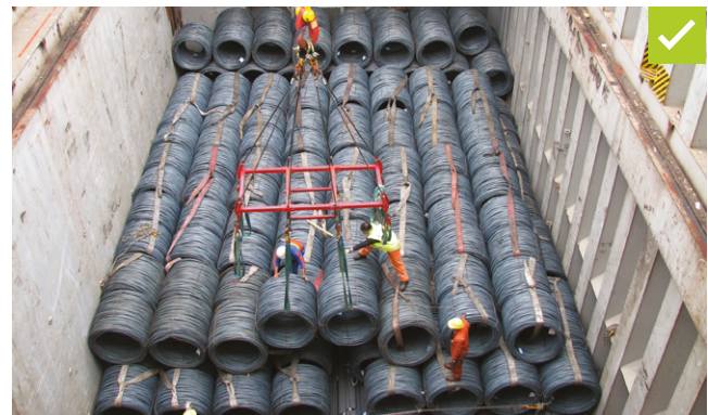
Figure 26: Coiled wire rod correctly stowed in a square hold
