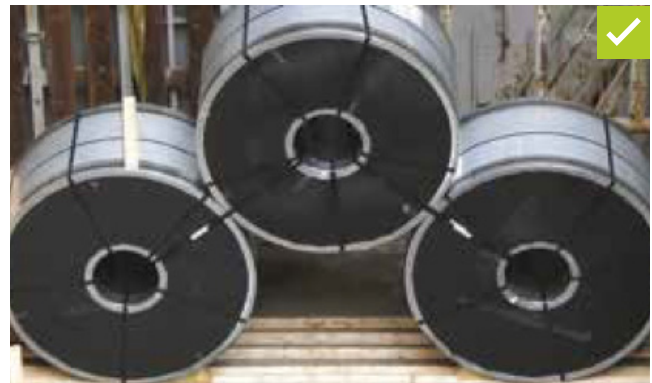
Figure 17: Coils correctly stowed with dunnage, wedges and a key coil
