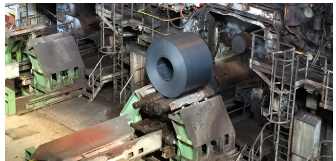
Figure 2: Hot rolled coil after rolling
