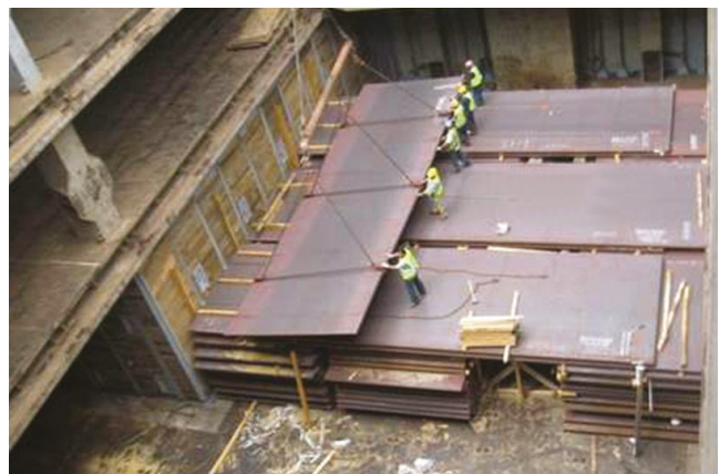
Figure 30: At sea, when conditions allow, check 'chocking and tommying'. Remember that cargo holds should only be entered after following your company's cargo space entry procedures and only when sea conditions allow working on deck
