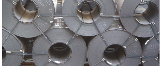
Figure 47: Coils stowed and lashed together with steel bands
