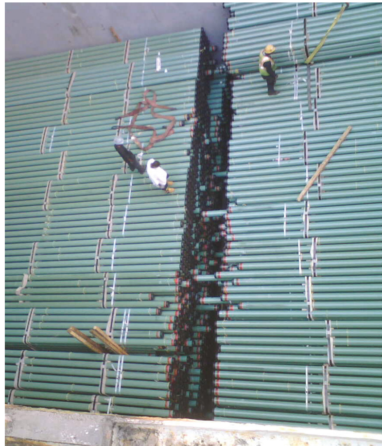
Figure 32: Bundles of coated pipes are stowed with vertical chocking
