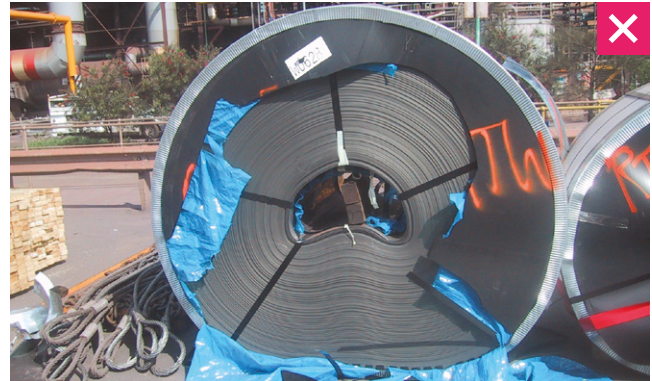
Figure 25: Cold rolled steel coil (CRSC) damage
