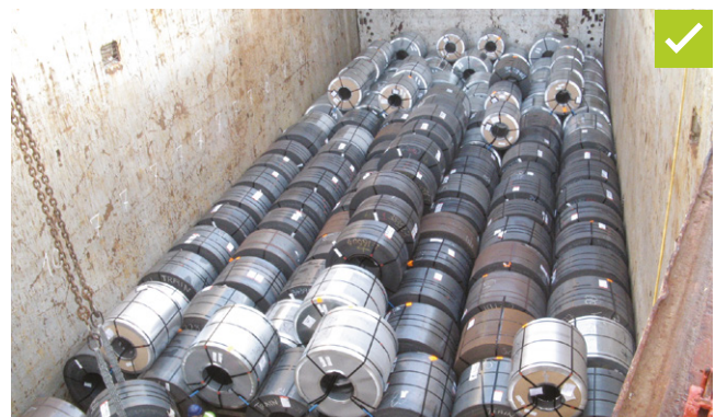
Figure 18: Coils tightly stowed with centre line key coils and multiple key coils fore and aft
