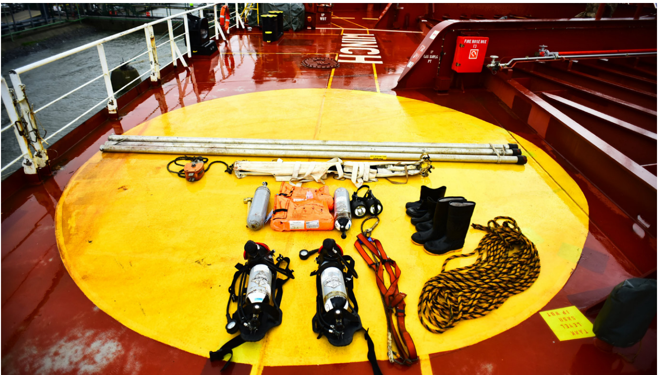
Figure 9: Safety and rescue equipment for entering an enclosed space
