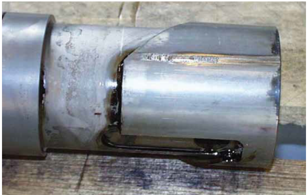
^ Fuel pump plunger scoring
